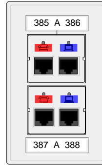
Work Area Outlet
